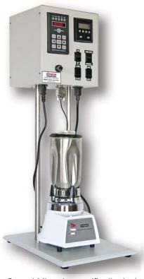
The M3080 Variable Speed Mixer is specifically designed to meet oil industry testing requirements. It functions as a mixer for cement and other shear-sensitive dry or fluid materials and complies with all existing API guidelines.
